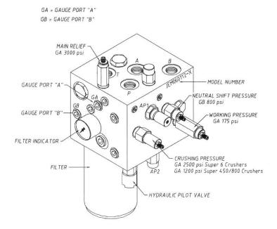
Install a 3,000 psi pressure gauge into the gauge port (GA) on the hydraulic block.
