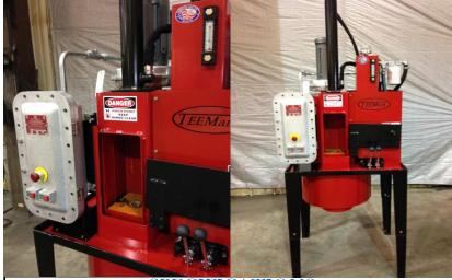
SPECIFICATIONS Crushing Force: up to 12,000 lbs Operating Cycle Time: 9 Seconds Dimensions: 90 inches high, 31 inches wide, 26 inches deep Shipping Weight: 900 Crushing Dimensions: 5-1/2 X 7 X 12-3/4
