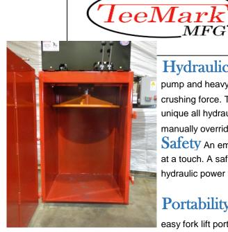
**Hydraulics** A rugged two-speed hydraulic pump and heavy duty cylinder to 37,000 pound crushing force. The ram is automatically cycled by a unique all hydraulic control valve. The cycle can be manually overridden at any point.
