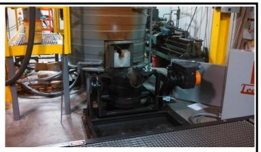
Here is a custom designed conveyor used to pour magnetic glass. The ladle is filled from the furnace and hydraulically moved to the conveyor where it is hydraulically tilted. This is all being done while the conveyor is moving. The system is set up with speed controls on all moving components for precision pouring. Final product is a sheet of glass.
