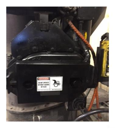
has developed a superior motorized tilt gearing package to provide uniform control and safety. The gearing utilizes the world renowned Baldor-Dodge gearing coupled with a Cone Drive Change Gear and a Baldor Brake Motor. To this we add a Right Angle Gearbox and a manual handwheel should power ever be lost.
